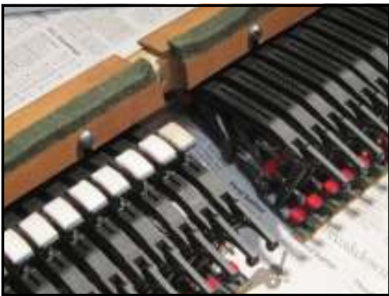
New composite parts being installed in a 125 yr. old piano = much time spent regulating.
