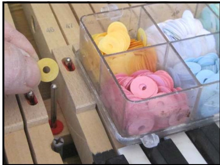
.03" inch paper punching being installed
