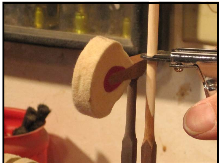
Newly spiced shank being cut to length.
